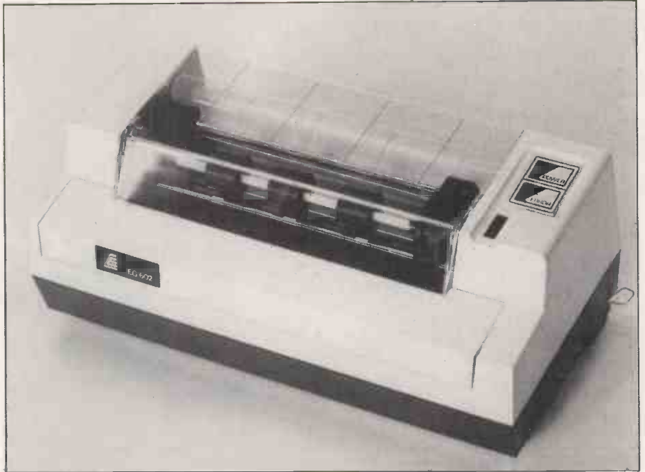
Eaca's EG-602 printer appears to be identical with the Seikosha GP-80 and prints graphics, lower case without descenders and double-width characters.
